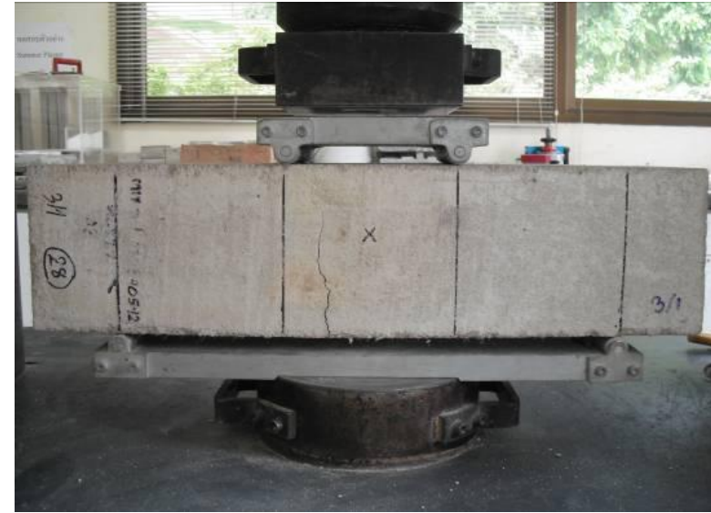
Steel Fiber Concrete W/C 0.45: Flexural strength 54 ksc (25 kg/m 3 )
