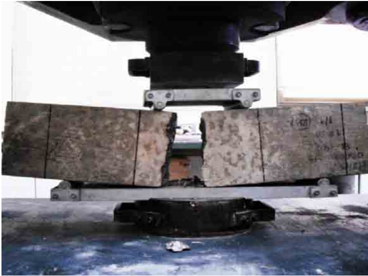
Normal concrete W/C 0.45: Flexural strength 47 ksc
